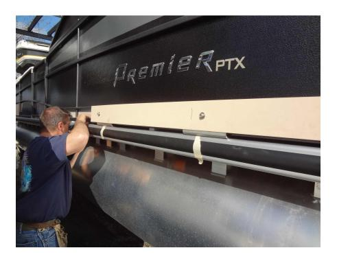
5. position the L brackets so that each bracket is over one of the aluminum beams running port to starboard. Drill thru the deck of the boat on the forward and aft sides of the beam, and use the aluminum backing bar to "clamp" the L bracket to the aluminum beam. (we do not recommend that you drill thru the aluminum cross beams of the boat) The arch will mount
