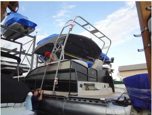
Your Pontoon Arch is open all the way around, so that wiring may be completely concealed inside. You may drill holes up to 1" in diameter for wiring entrance and
