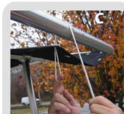
Pull folded end of line through about 6".
