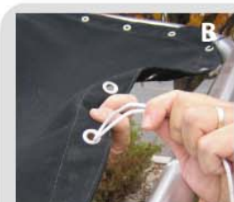
Fold length of line in half, and put over the pipe and through eyelet.
