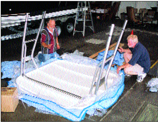
■ STEP 2: After lifting the top from its shipping frame (a two-man job), we carefully cut away the protective shrink-wrap. We saved the shipping blankets. These came in handy later.
