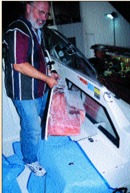
■ STEP 4: To gain access for through-bolting the hardtop mounts, we removed the side panels of the 2460 Denali. To prevent accidentally tearing the seats, we also removed most of the upholstery, then put down the shipping blankets to protect the rest of the interior.
