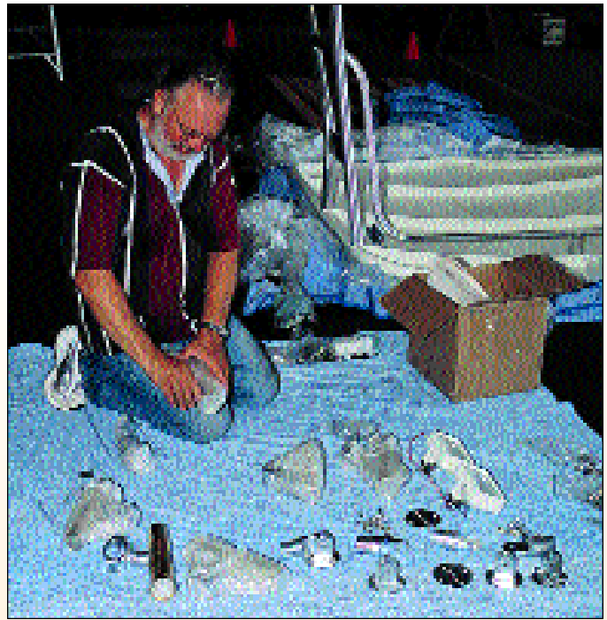
■ STEP 3: Universal mounts (lower right foreground) are included with the hardtop — but not mounting bolts, nuts and washers. We also ordered some accessories, such as rod holders and spreader lights.
