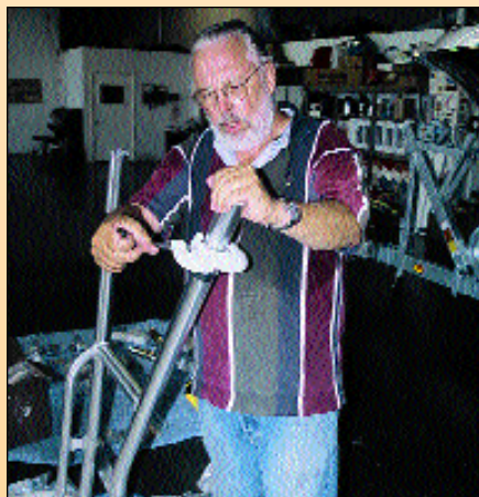
■ STEP 6: Using a pipe cutter, we removed 4 to 6 inches of excess length (used to bolt the top to the shipping frame) from each of the four legs. ►
