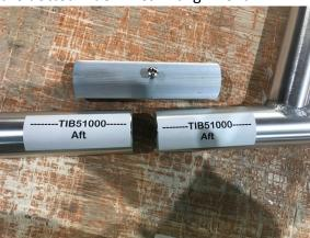
Epoxy cures very quickly, there is 10 to 15 minutes of work time depending on temperature. Applying Epoxy to the inside of pipes will minimize excess squeezed out during assembly. Promptly clean any excess before it completely cures
