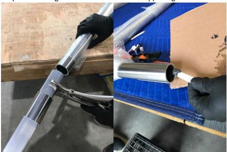
Epoxy the lower section of the leg and tap into place with soft mallet or block of wood. Keep index marks on labels aligned
