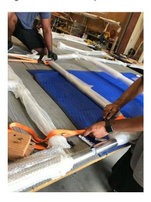
If your T-Top has rod holders, make sure the orientation is correct, Rod Holders "UP", forward section of T-Top turns down.
